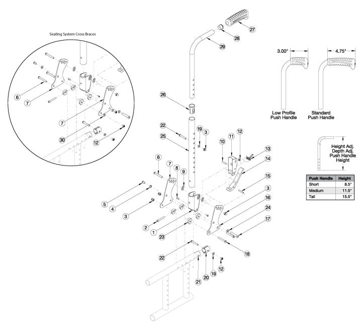
This backrest style was released February 8th, 2021 Low Profile Push Handles are not available with Heavy Duty Option or Drum Brake If the Drum Brake is present, see Drum Brake page for back Cane replacements If Anti-Rollback is present, see Back Tubes for Anti-Rollback System
