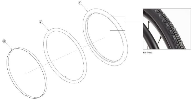
Please note tab mounted handrims must be installed prior to the tire being installed.
