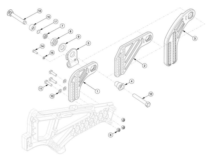
Effective 2/8/2023: axle receiver part number 003300 has been replaced with 115908. If changing from 003300 to 115908 a new washer and nut are needed.
