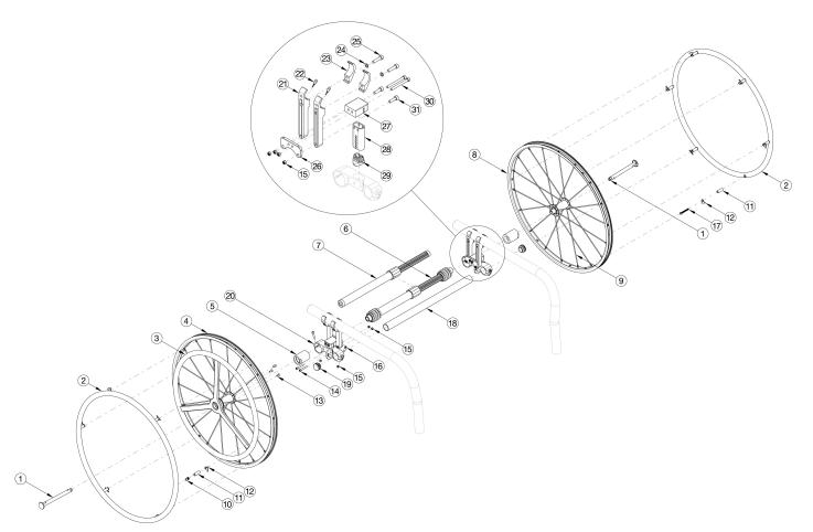
If retrofitting to add the One Arm Drive, new rear towers are required in addition to the complete One Arm Drive system and camber tube kit. Effective 5/13/2022, all One Arm Drives will be shipped with a close mounted handrim on the non-drive wheel. Most One Arm Drive kits do not include rear tires. Tires need to be quoted separately. Used on Rogue XP chairs invoiced starting on 3/12/25
