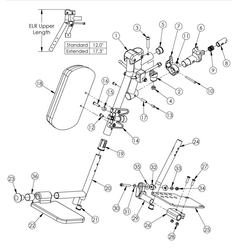
Small composite footplates are used on 14-16" seat widths. Large composite footplates are used on 17-22" seat widths. Sizes for assemblies are based on seat width with straight frame; if Tilt chair has Offset Frame, add 2" to seat width. For a complete Elevating Leg Rest with Heel Loops or 4-Way Latch, select an upper assembly and the desired extension tube and footplate assembly from the Elevating Leg Rest page.
