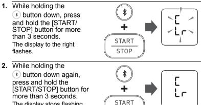
The display stops flashing, then your monitor is restored to the default settings.
