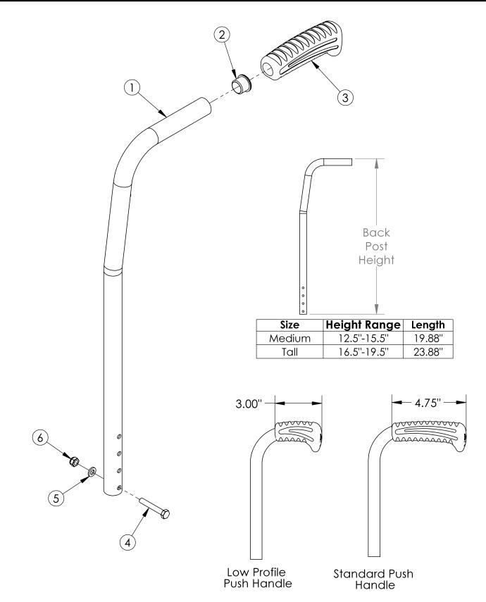
Low Profile Push Handles are not available with Heavy Duty Option or Drum Brake If changing from another style backrest and the Drum Brake is present, a new Drum Brake Cable Kit may be required If Anti-Rollback is present, see Back Tubes for Anti-Rollback System
