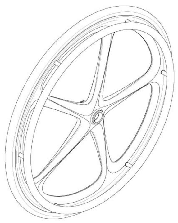
Not all components of the Wheel, Tire and Handrim kits will be listed. If changing wheel size and anti-tips are present, new anti-tips may be required. If changing wheel size or style, new axles, receivers, and/or axle plates may be needed. See Liberty Axles page for axle and receiver utilization.
