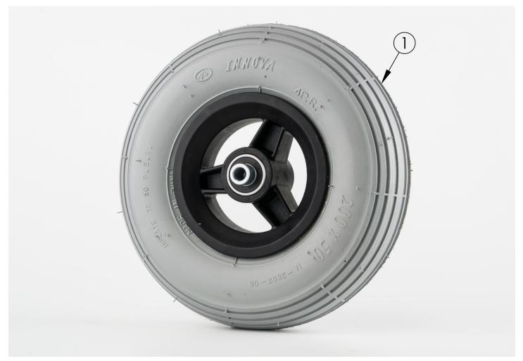
If retrofitting, new forks and hardware may be needed. Spacers are built in to 8" x 2" casters. Additional spacers are not needed. If changing size of casters, new forks may be needed.
