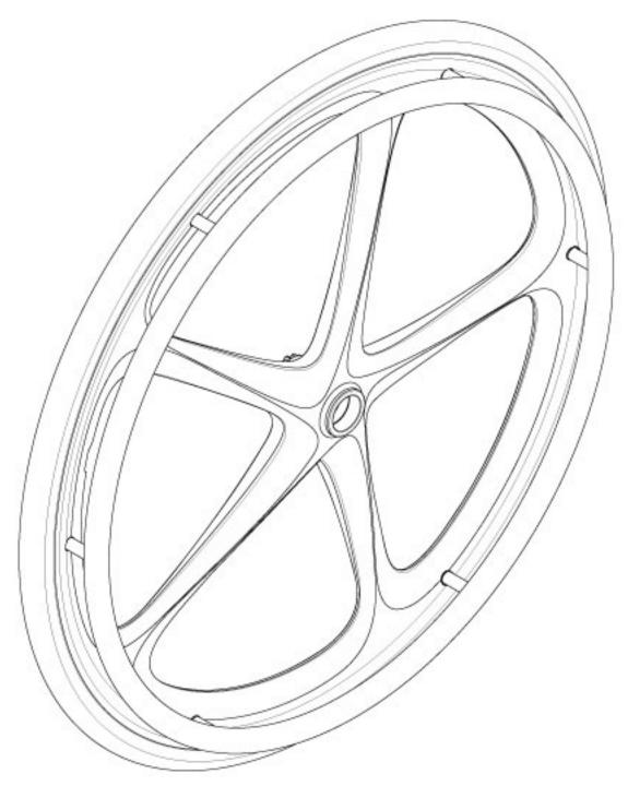
Not all components of the Wheel, Tire and handrim kits will be listed. If changing wheel size and anti-tips are present, new anti-tips may be required. If changing wheel size, new axles/receivers and handrims may be needed. If changing wheel size and Attendant Foot Lock or T-Arms are present, spacer 112503 is required which can be found on the CR45 Axle Plate page. See CR45 Axles page for axle and receiver utilization.
