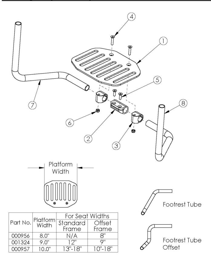
For attaching footrest hardware, reference the Clik Side Frame pages (serial numbers CLK005270 and after) or Discontinued Side Frame pages (serial numbers prior to CLK005270) If changing width of chair, new footrest tubes are required.
