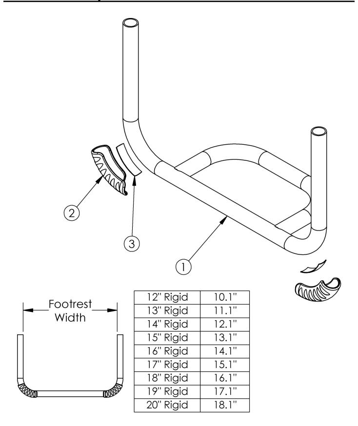
Use Short Footrest if 0" taper and footrest length is 9" - 10.5" or if 1" or 2" taper and footrest length is 9" - 15.5" See Ethos Seat Frame page for hardware to attach footrest tubes to chair.
