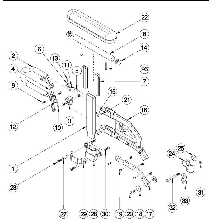
Short Side Shield used with 14"-17" Seat Depths. Long Side Shield used with 18"-20" Seat Depths If retrofitting, Receivers are needed. If retrofitting to Height Adjustable Flip Back T-Arms and One Arm Drive is present, a new drive shaft may be required. In addition to a new drive shaft, order the corresponding hardware kit: 109438 for Blade Style One Arm Drive, 503433 for Hex Style One Arm Drive or 112898 for Quick Release Style One Arm Drive
