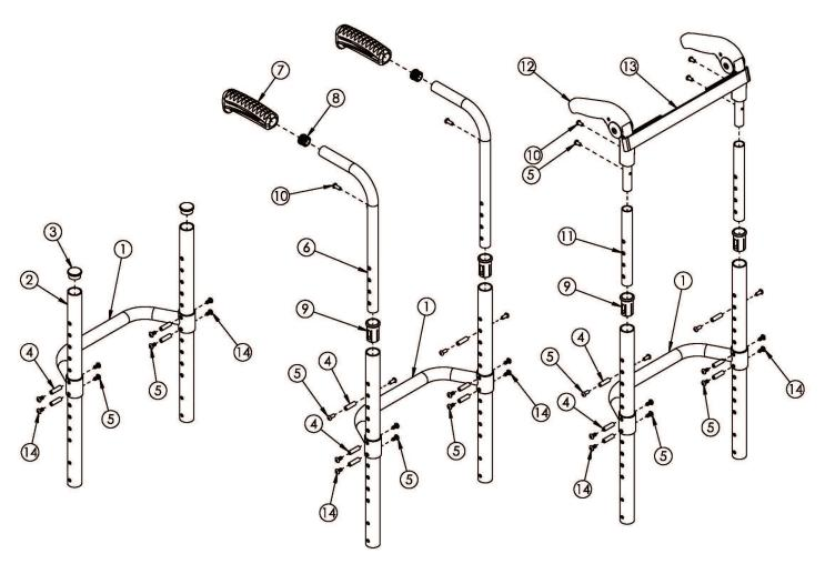
If chair was ordered with Rigid Locking Fold Down Back, please see Rigid Fixed Height Back Post with Adjustable Height Rigidizer Bar page. Effective on Rogue starting with serial number RG0016612. If retrofitting to this backrest on Rogue, a new backrest mount and hardware may be required. Tension Straps (#13) are based on seat width and used in combination with back upholstery.
