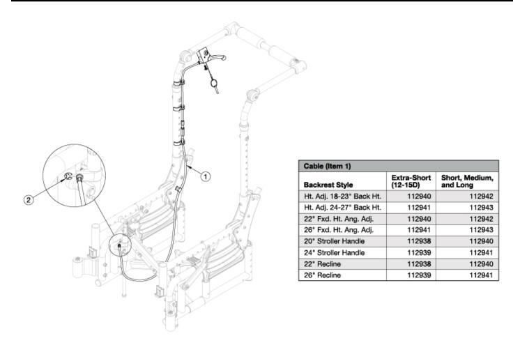
Is your depth changing? Will your existing tilt cables achieve your new depth? If no, please select the appropriate tilt cable based off your new configuration on the table above. Each cable kit contains two cables and two e-rings.
