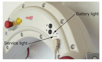
If the lifter is run up and down constantly for a longer period, the electronics may be overheated, and then the lifter will stop. The service diode will give a yellow flashing signal until the lifter has cooled down sufficiently to work again.
