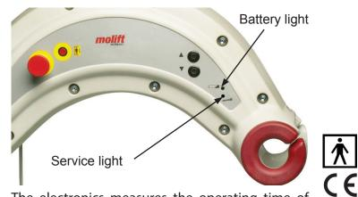
The electronics measures the operating time of the lifter, and after a specific time the yellow light will illuminate, indicating that the lifter needs service. Take contact with your local Molift service representative/dealer. The lifter can still be operated, but after a while an audible alarm will sound, to remind the operator that the lifter needs service immediately.
