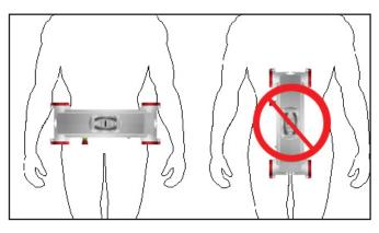
When using slings intended for two point suspension, the suspension shall be used diagonally, i.e. loops from the sling shall be fastened on hooks diagonally opposite.
