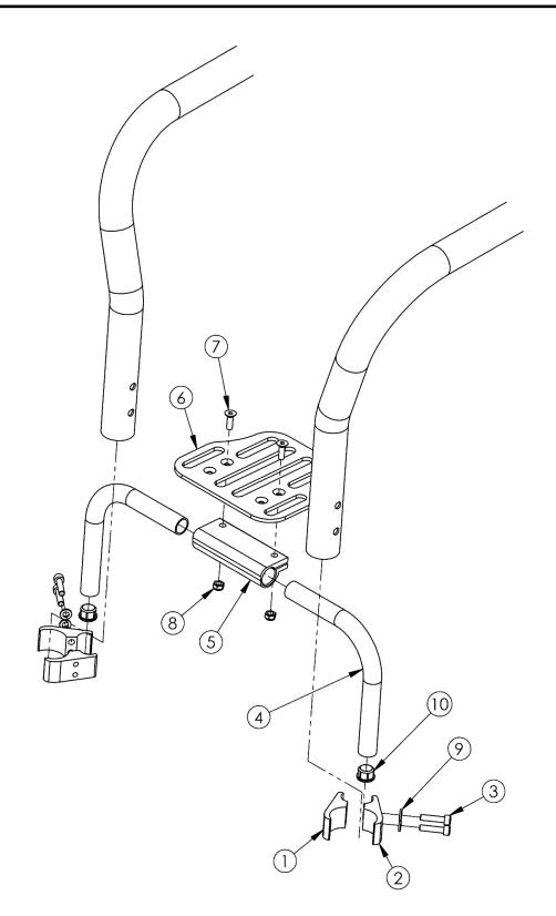
Footrest assemblies based on straight frame Used on serial numbers prior to TS010953, TSHD003973, TSTR004735, RGXP008523, RG0018443
