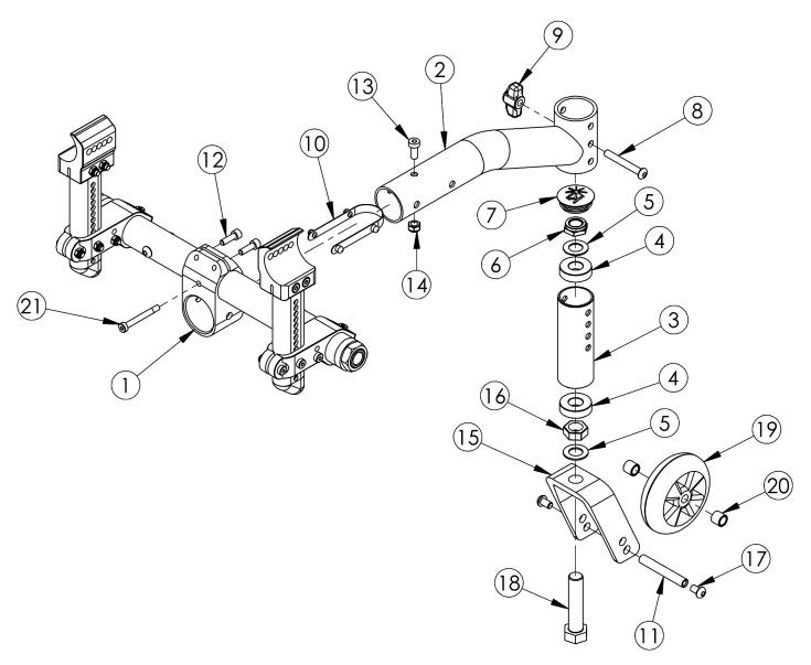
A new camber tube is needed if retrofitting to the Standard 5th Wheel
