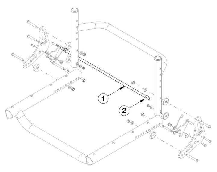
Utilize this page if chair has Locking Fold Down Back (Rogue 10 Style). Backrest Release Bar based on seat width. This Tsunami Backrest Mount and Hardware is only used with the Tsunami Style Backrest.
