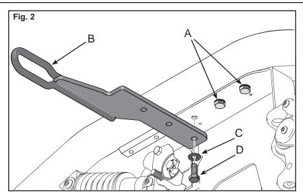
3. Now remove the remaining two screws and swing the transit bracket into place. Install two more supplied 5/16 x 1 Hex Head Screws (D) using the original washers (C). Torque all three screws to 27-35 ft-lbs. (Fig 3) Reinstall the Drive Wheels and repeat the process for the opposite side.
