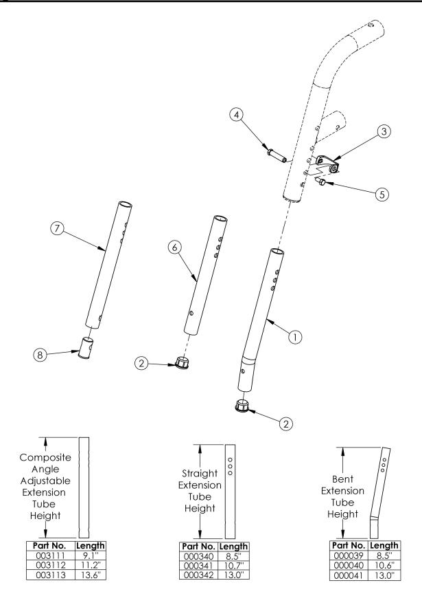
If hangers are being quoted/ordered in addition to extension tubes, fasteners (#3, #4, #5) are already included with the full hanger assemblies (Reference the 60,70,80,90 degree hanger pages).
