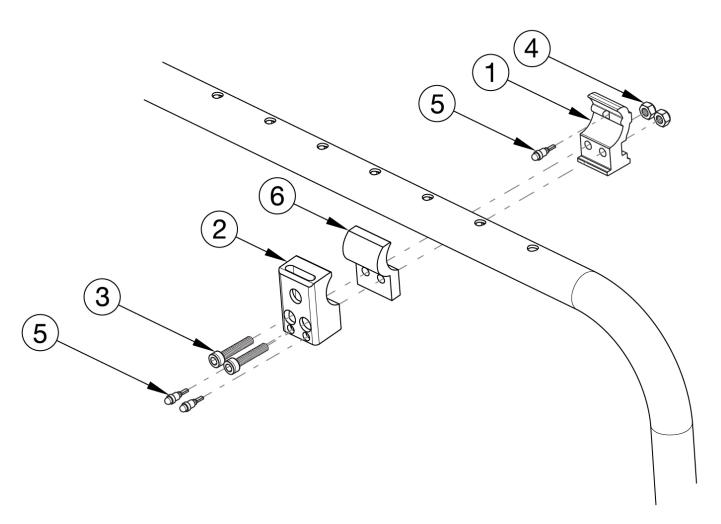
Color anodized versions of this receiver may not contain the two counterbored holes at the bottom of the receiver
