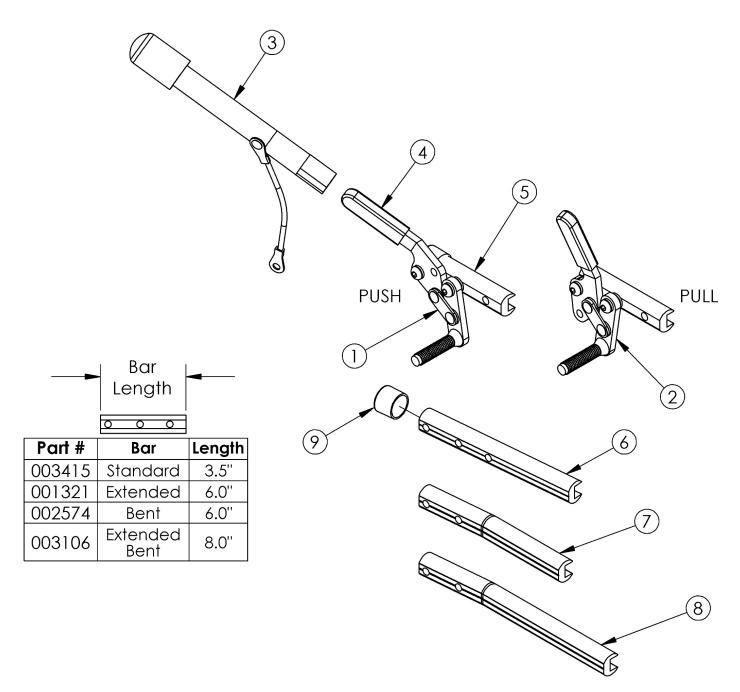
Please confirm wheel lock bar length and style for correct replacement parts
