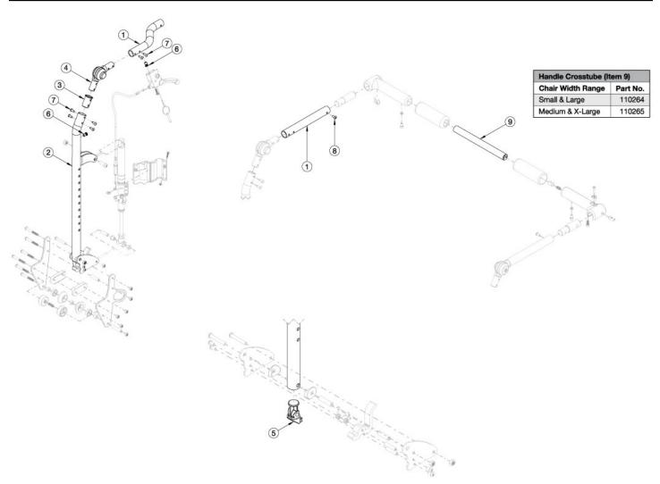
Callout #1: 10"-13" widths receive the curved tube and 14"-18" widths receive the straight shaped tube. When changing backrest types, check to see if new cables and tilt triggers are needed for both foot and hand tilts.
