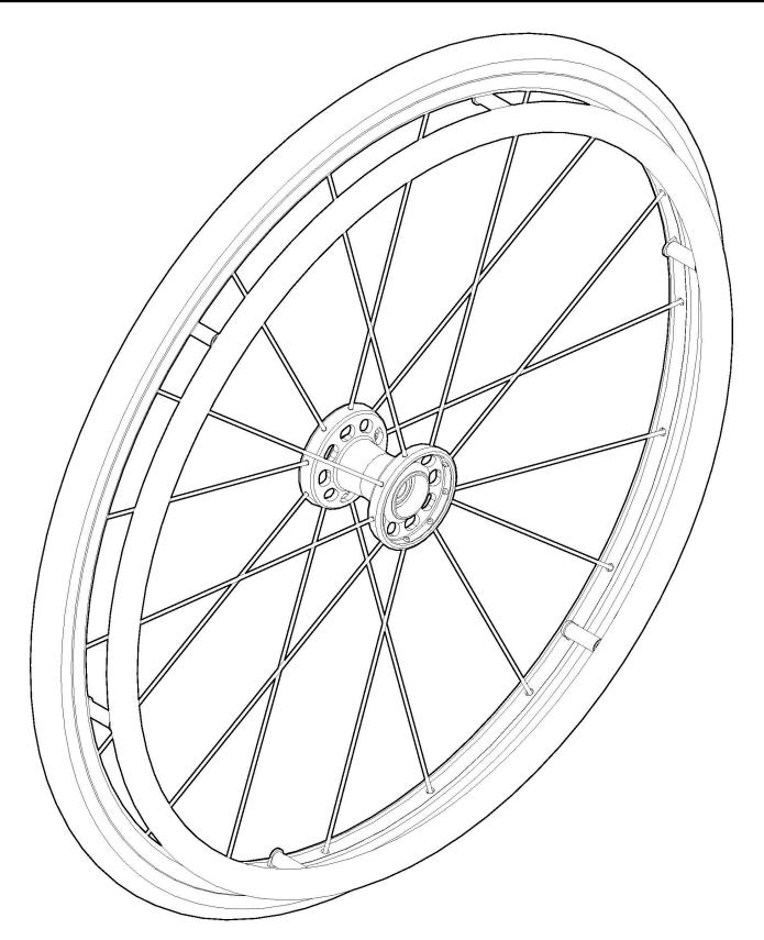
Not all components of the Wheel, Tire and Handrim kits will be listed. These kits cannot be used if Drum Brake is present. If changing wheel size and anti-tips are present, new anti-tips may be required. If changing wheel size or style, new axles may be needed.
