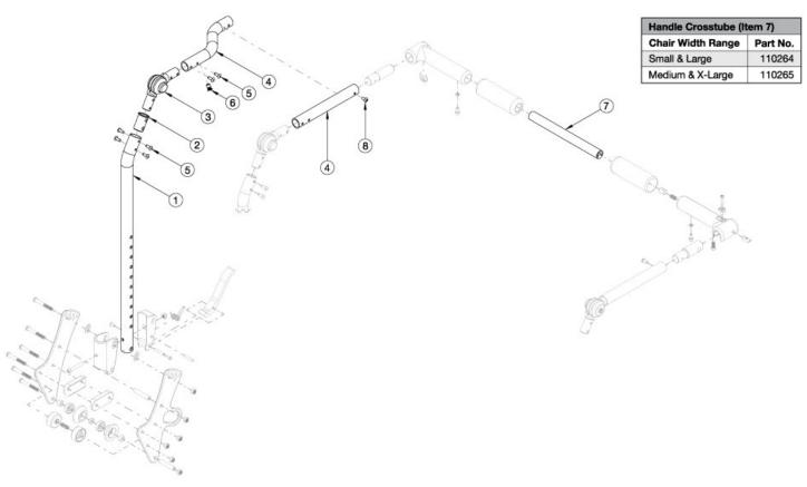
Callout #21: 10"-13" widths receive the curved tube and 14"-18" widths receive the straight shaped tube. When changing backrest types, check to see if new cables and tilt triggers are needed for both foot and hand tilts. If chair was invoiced prior to 12/18/23, an upper back tube assembly is required. If chair was invoiced after to 12/18/23, upper back tube assembly parts can now be purchased individually
