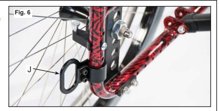
11. Adjust the Transit Bracket Assembly (J) so the measurement from the top of the front upright frame tube to the top of the Transit Clamp (A) is 5 1/2" (Fig 7).
