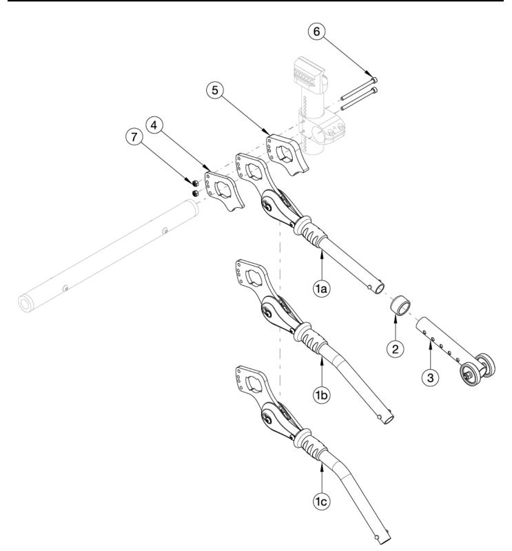
Contact Customer Service for chairs with more than 2" of variance between Front and Rear Seat Height. Complete assemblies contain "one" complete user activated anti-tip. Quantity two is required for a pair. A pair of User Activated Anti-Tips is not available if a tipping lever is present
