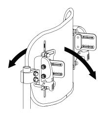
3 Tighten all hardware to 110 in-lbs except the acom nuts which are tightened to 80 in-lbs. Overtightening the back post clamp hardware may cause damage to backrest canes.
