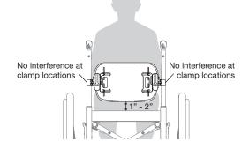
Adjust backrest so it appears centered between the two back canes and both clamps are set at the same height on both sides. Using a tape measure is recommended to ensure both sides are set up equally.
