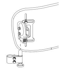
Visualize the user seated on the chair with a cushion and where the clamps will mount on the backrest canes. Ensure there will be no interference with the backrest canes. The bottom edge of backrest will typically fall between an 1" to 2" above the top of the cushion. Loosen the mount clamps and install onto backrest canes.
