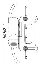
2 The angle and the depth of the backrest are adjusted, if needed, at the same time. Loosen the two bolts on the bracket and adjust the angle and depth of the backrest in one movement. Retighten hardware once desired configuration is achieved.
