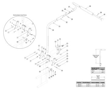
This backrest style and removable stroller handle extension was released February 8th, 2021 If changing from another style backrest and the Drum Brake is present, a new Drum Brake Cable Kit may be required If Anti-Rollback is present, see Back Tubes for Anti-Rollback System
