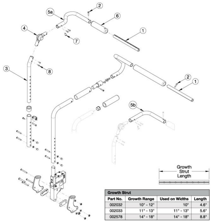
Has your width changed? Will the push handle (#5) and growth strut accommodate your new width? If no, please select the appropriate upper back tube assemblies and growth strut.
