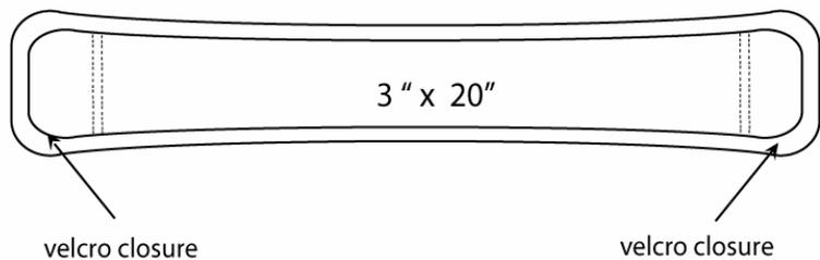
Figure 2: Front view of Compression Straps (4 per harness)
