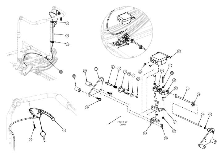
This design effective starting with serial numbers FCR0026599 and FCHD002333. If serial number is prior to FCR0026599 and FCHD002333 new upper back cane assemblies are required in addition to the hand tilt mechanism. If drum brake present see that page for trigger replacements. If drum brake present, see drum brake page for replacement parts.
