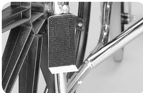
Fig. 1 Wheelchair Mount attached to lower, rear wheelchair frame
