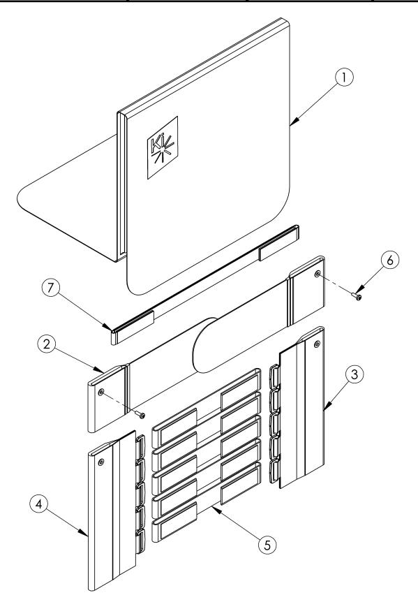
Tension Straps (7a-7d) are used with the combination of Fold Down Push Handle and Tension Adjustable Back Upholstery. Tension straps (5a-5d and 7a-7d) are based on chair width. Backrest cover kits with two straps and Tension Adjustable assemblies include Installation Instructions.
