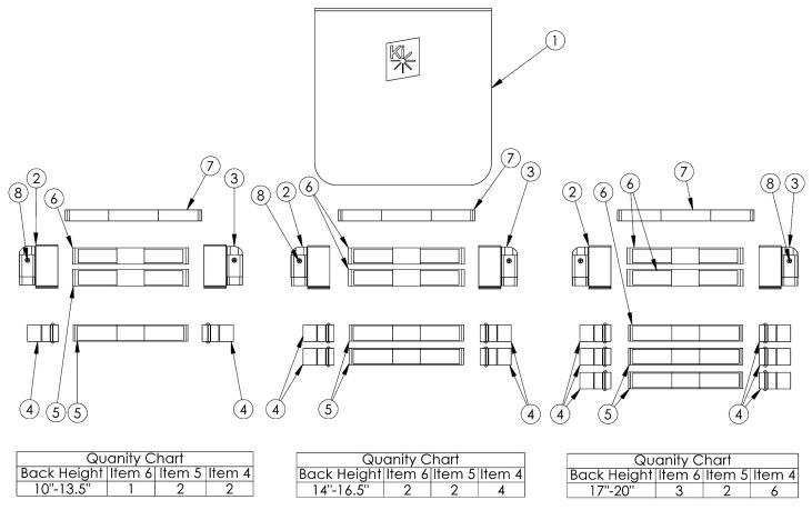
Open Back Panels are used when integrated push handles are present. Closed Back Panels are when backposts without push handles are present. Tension Straps (7a-7d) are used with the combination of Fold Down Push Handle and Tension Adjustable Back Upholstery. Tension Straps 6a - 6f and 7a - 7d are based on chair width.
