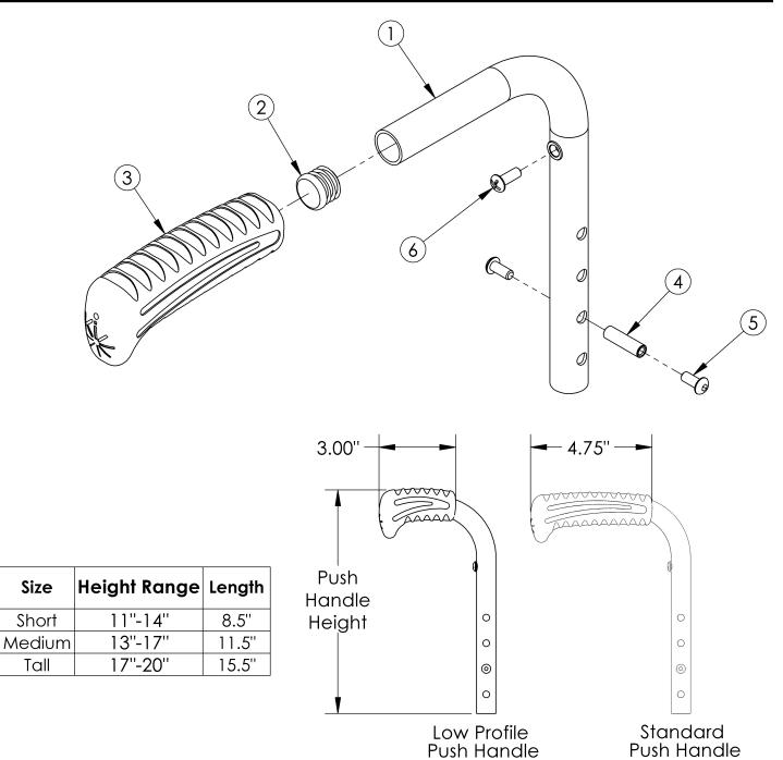
The above chart is in reference to the height adjustable back post w/ push handle If changing from another style backrest and the Drum Brake is present, a new Drum Brake Cable Kit may be required
