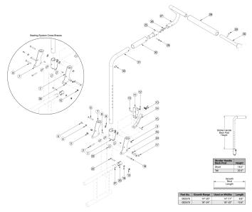
This backrest style and removable stroller handle extension was released February 8th, 2021 If changing from another style backrest and the Drum Brake is present, a new Drum Brake Cable Kit may be required If Anti-Rollback is present, see Back Tubes for Anti-Rollback System
