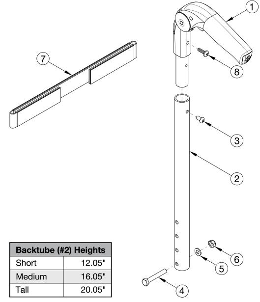
Tension Straps are used with the combination of Fold Down Push Handle and Tension Adjustable Back Upholstery. Straps are based on chair width. Not available with Heavy Duty Option If Anti-Rollback is present, see Back Tubes for Anti-Rollback System
