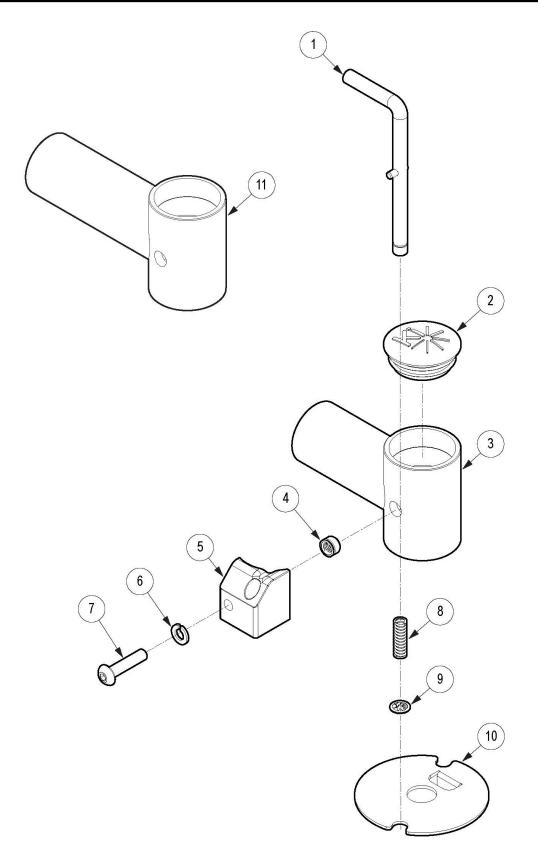
This design effective starting with serial numbers TS010961, TSLW003890, TSHD003974, TSTR004740 and RG0018469 To retrofit from previous Caster Pin Lock design, you will need new caster housings, caster lock mounting blocks and M5 split lock washers. If retrofitting to add Caster Pin Locks, you must order an assembly that contains caster housings.
