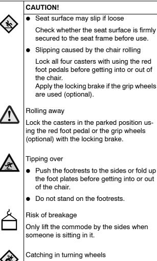
When using the optional grip wheels, do not grip between the spokes or between the seat frame and the turning wheels.
