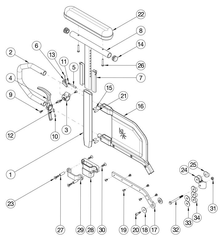
If retrofitting, Receivers are needed. Short Side Shield used with 14" - 17" Seat Depths. Long Side Shield used with 18" - 20" Seat Depths. If retrofitting to Height Adjustable Flip Back Tall T-Arms and One Arm Drive is present, a new drive shaft may be required. In addition to a new drive shaft, order the corresponding hardware kit: 109438 for Blade Style One Arm Drive, 503433 for Hex Style One Arm Drive or 112898 for Quick Release Style One Arm Drive.
