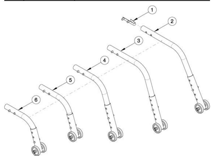
If changing to or from a reclining configuration, new sized anti-tips may be required. If retrofitting, Anti-Tip Receivers are needed.
