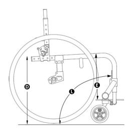
FRONT ANGLE L Measure from frame front to floor.
