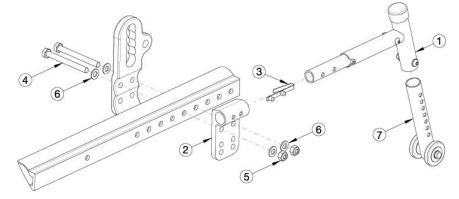
Anti-Tip assemblies are based on rear wheel size. Anti-Tip Receivers are installed on Focus chairs. Receivers are not needed when retrofitting anti-tips to a chair unless removing the Vent Tray and replacing the Vent Tray Anti-tips with the Focus CR Rear Anti-tips.
