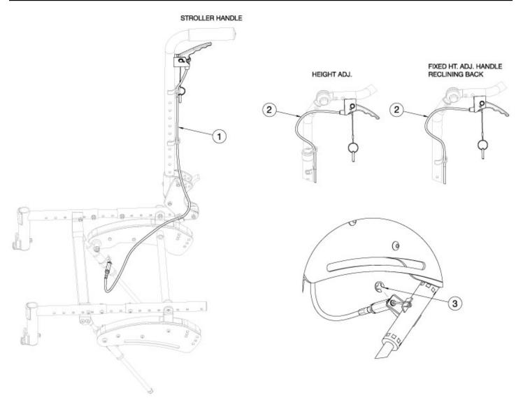
Has your depth changed? If yes, please review the notes below the tilt cable part numbers to determine if a new hand tilt cable is necessary.
