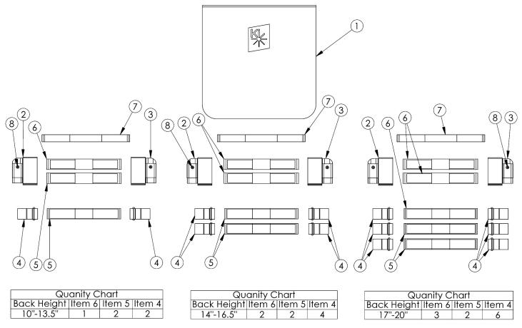
Open Back Panels are used when integrated push handles are present. Closed Back Panels are when backposts without push handles are present.
