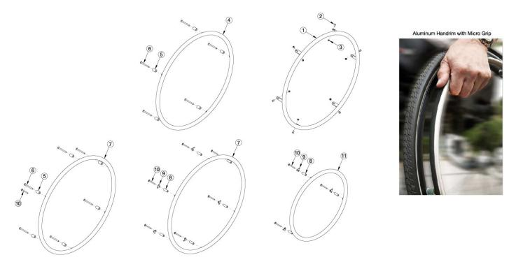
For more information see Handrim Hardware Chart. If replacing handrims use Aluminum Anodized Handrim Reference to match style. Quantity in Handrim Hardware Kits are for one wheel. Tab mounted handrims must be installed prior to the tire being installed.
