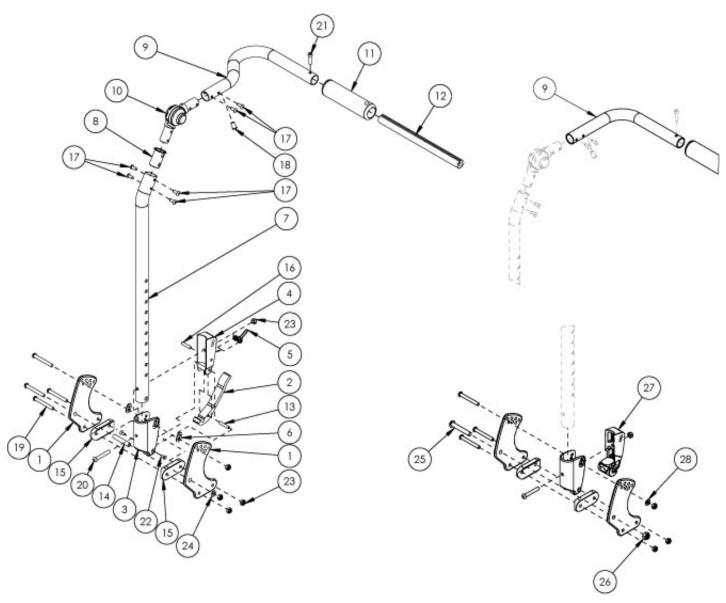
Callout #9: 10-13" widths receive the curved handle and 14-18" widths receive the "L" shaped handle.
