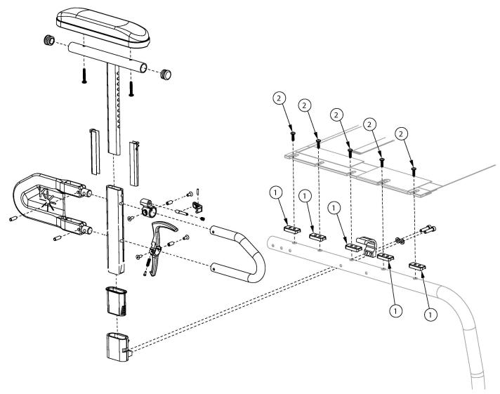
If Height Adjustable T-Arms are present, depending on change in depth, seat rail saddles and attaching hardware may be required
